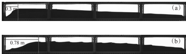
图7 聚丙烯酰胺溶液(a)和全悬浮压裂液(b)的最终砂堆形态 Fig.7 Final sand pile morphology of polyacrylamide solution (a) and fully suspended fracturing fluid (b)
